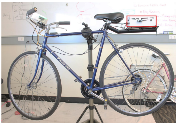
Figure 1. Instrumented bicycle with sensors identified.
