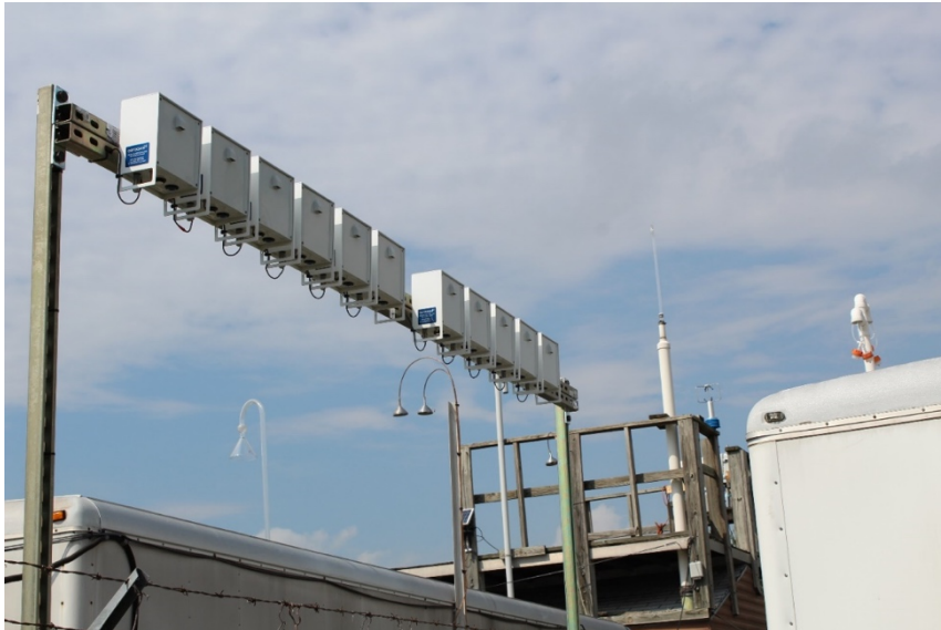
Figure 1: 12 Aeroqual AQY Version 1 (AQY1) low-cost air quality monitors co-located at the Hinton site in Dallas.
