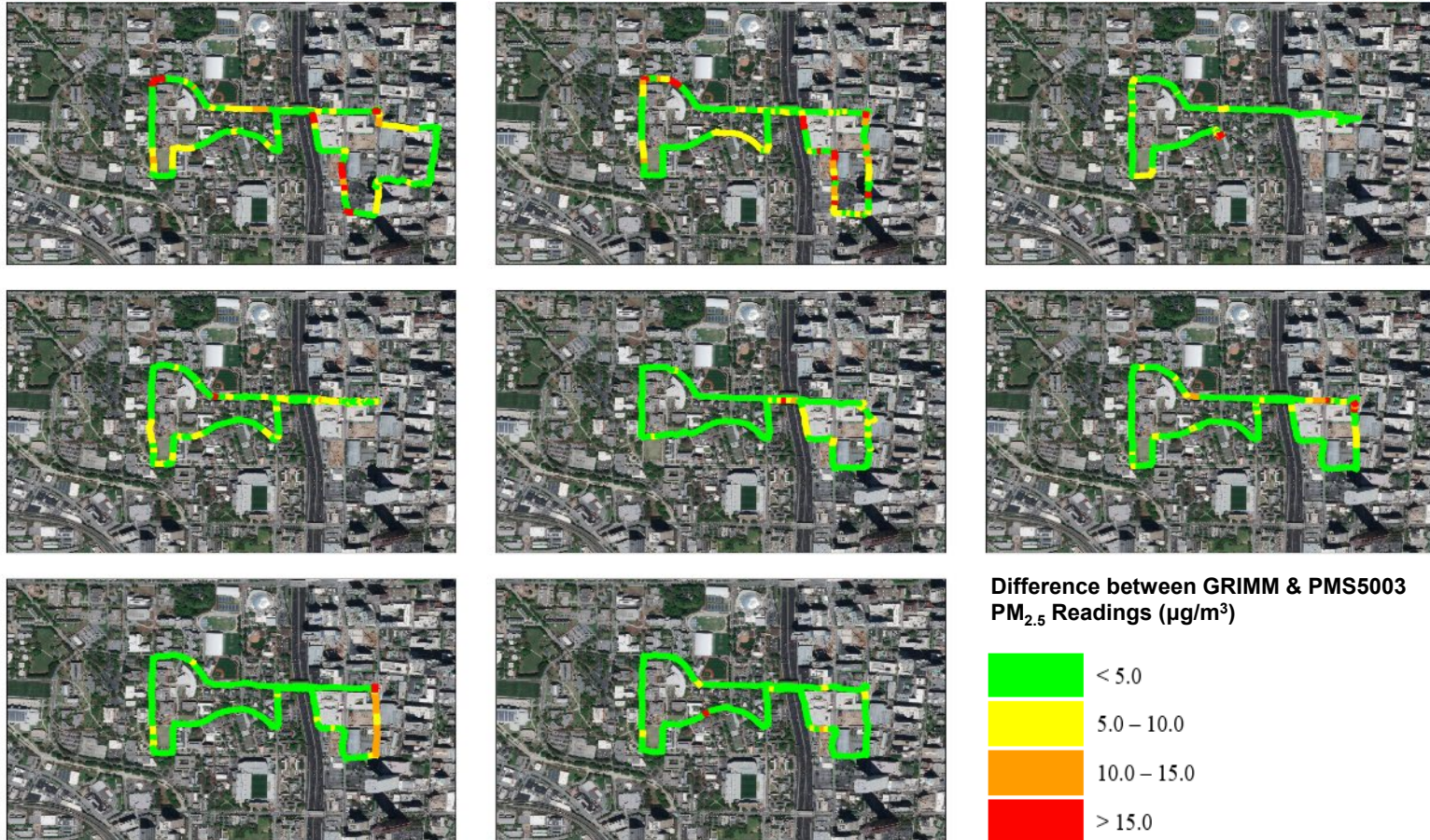
Difference between GRIMM 1.109 and PMS5003 sensor readings during mobile monitoring
