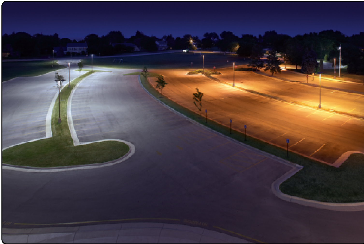
Side by side parking lots lit by LED and HPS lights ( LED outdoor area lighting fact sheet , 2008).
